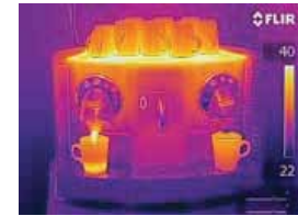
MSX allows seeing even more detail on the thermal image.
